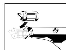
4. On completing the application, move the plunger back again by pressing on the release button and lift the application capsule out.
