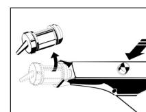
5. Disinfect the applicator after each use. Conventional disinfectant wipes or solutions can be used for disinfection. The Omnident C Applikator can be steam sterilised at up to a maximum of 134 °C (steam steriliser, follow manufacturer's instructions).
